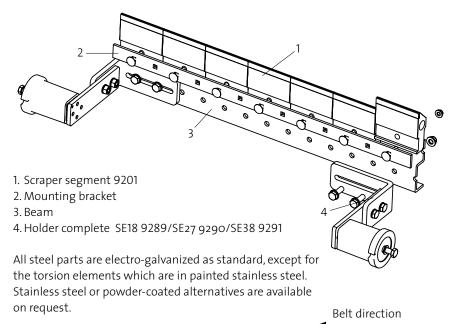
The scraper blade is made of PU with a carbide edge.
